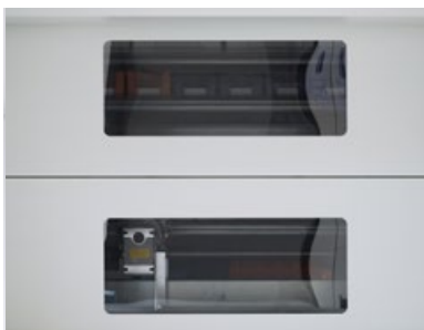
The integrated inspection windows of the shutter doors offer the view on the movement of tray and extractor device.
