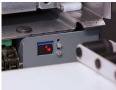
The built-in retro-reflective sensor for the tray detection saves maintenance costs and lowers installation effort.
