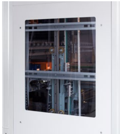
The inspection windows on both sides of the tower allow external control of trays and extractor device.
